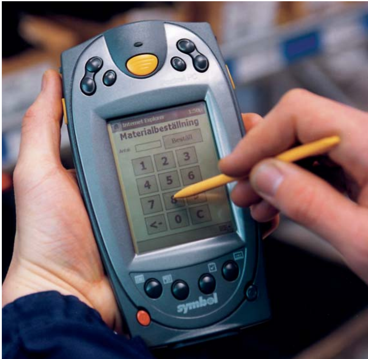
Hand-held computers with a wireless LAN are used to make the handling of materials at the plant faster, safer and more efficient.
